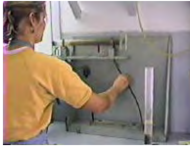
Manually-Operated Shaker Figure 4
