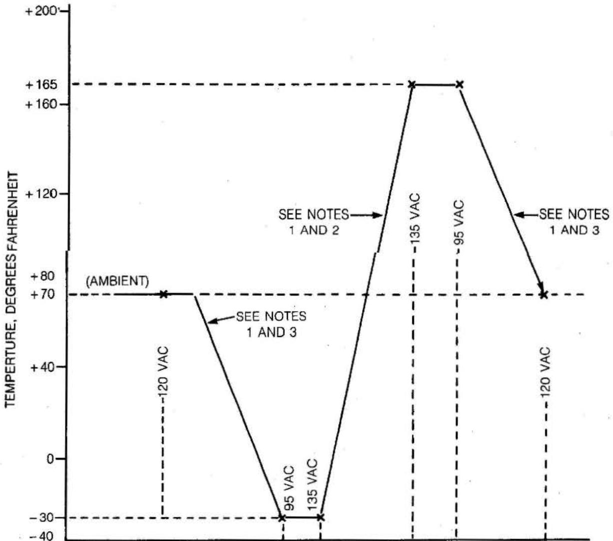
NOTE 1 – The rate of change in temperature shall not exceed 30°F (18°C) per hour.
