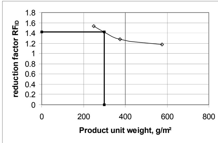
Figure, A-2. Example interpolation of  $RF_{ID}$  from damage measurements on products from the same line but with different weights. For a product of weight  $300 \text{ g/m}^2$ ,  $RF_{ID} = 1.42$  (Note:  $1 \text{ oz/yd}^2 = 0.0295 \text{ gm/m}^2$ ).
