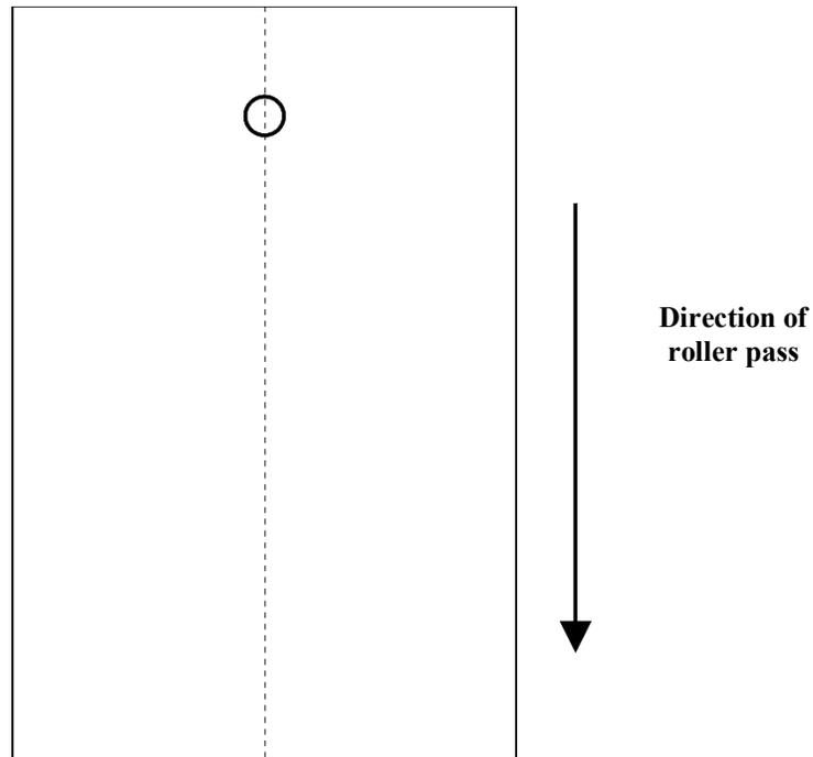
**Method B****Footprint of the gauge test site**
