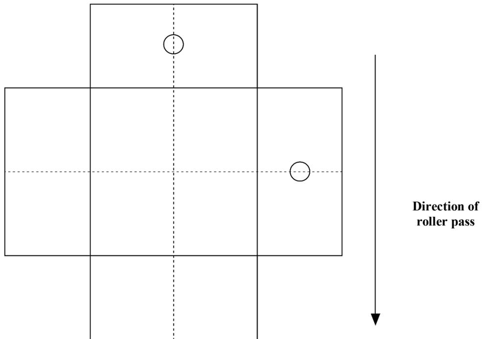
**Method A****Footprint of the gauge test site**
