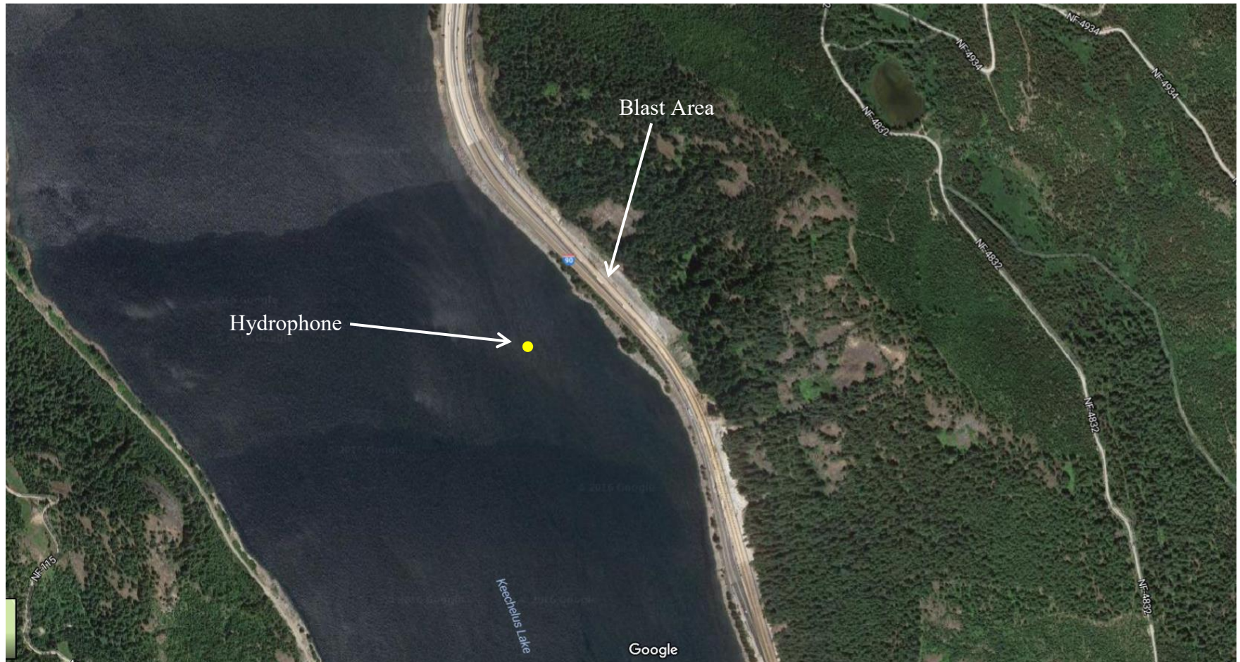
Figure 2: Hydrophone location relative to the upland blast area
