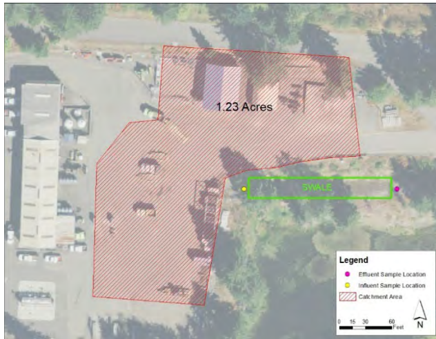
Figure 7. Mottman CABS monitoring site and associated drainage area
