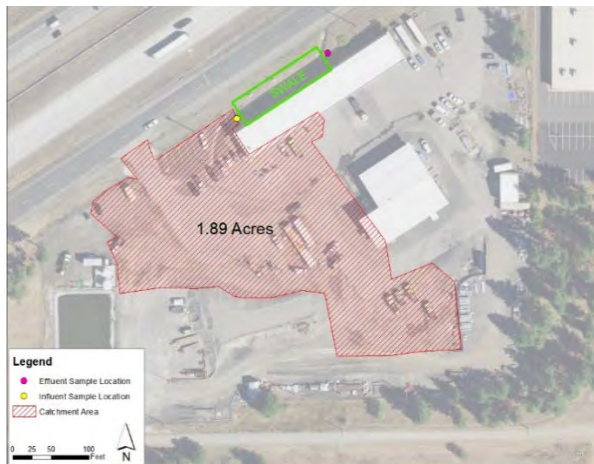
Figure 9. Geiger CABS monitoring site and associated drainage area
